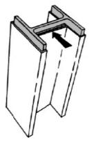
6) As each section is installed, lap as shown until the desired length of the pile is covered.
