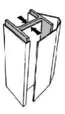
4) Continue to wrap the iacket around the balance of the uncovered pile section, squaring up the flange edges in the process .
