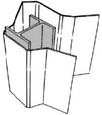
1) Center flange cover section of jacket over outside of pile flange (starting either side of pile).
